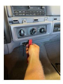
2. Remove the two 7 mm climate bezel screws and pry out to remove the bezel.
