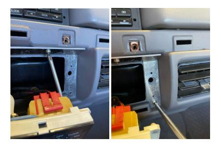
7. Re-install the climate control assembly to the OBS Solutions bracket and re-install the climate control bezel and dash trim piece.
