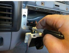
5. Remove the OBS Solutions climate control bracket. Using a ⅓ inch drill, drill out the marked area. (We like to use a pic tool that we head up and pierce the marked locations. We find this is a great alternative to drilling).
