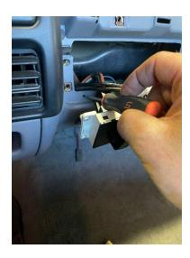
6. Re-install the OBS Solutions climate control bracket and install the four phillips screws that were provided into the four 11/64 holes.
